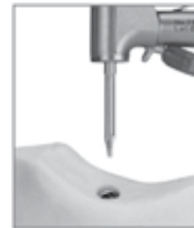
Insert Tap In Dimple & Use In REVERSE
